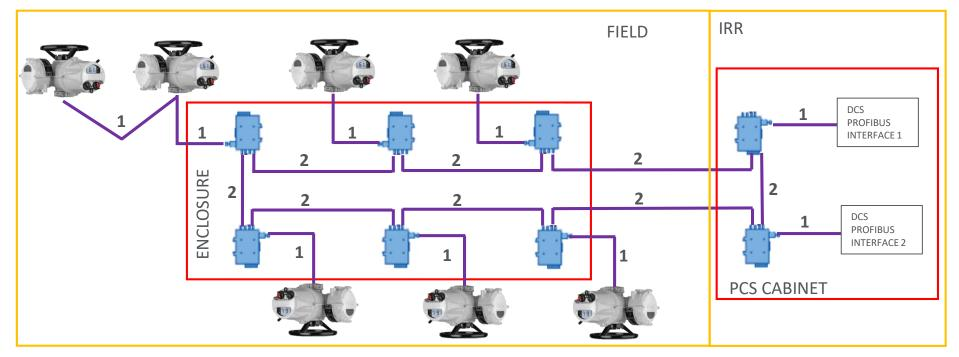
The fault of one OLM would cause the lost of one segment.
