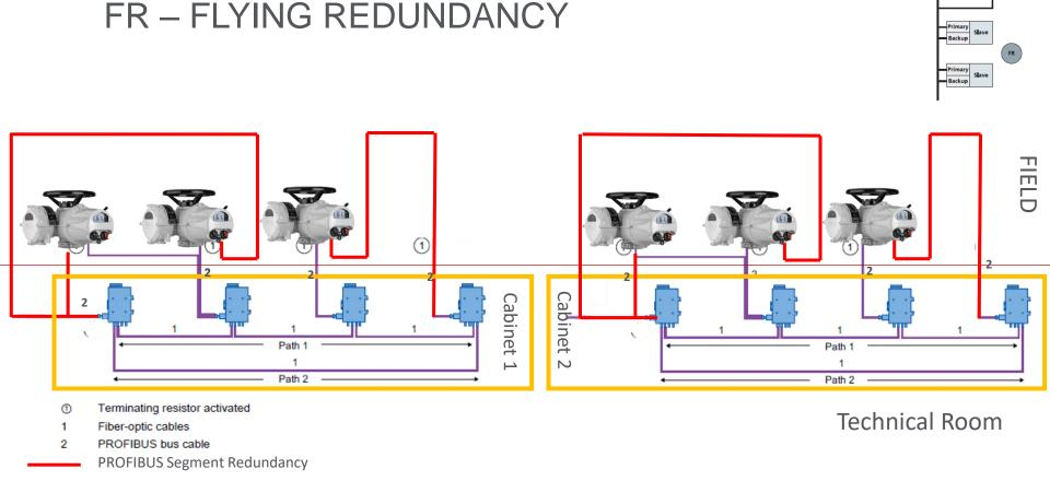
This configuration also allows to fit all the OLMs in two Cabinets located in the Technical Room. The FO installation and ring is confined inside each cabinet but the redundancy is ensured by both OLM Rings and Profibus Segments Redundancy.
