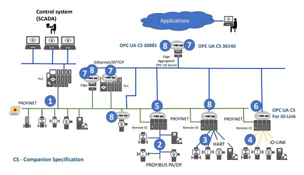
Figure 18: Information flows in an exemplary topology structure
