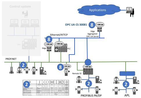
Figure 29: Typical integration variants of process equipment (PA devices) in the communication network
