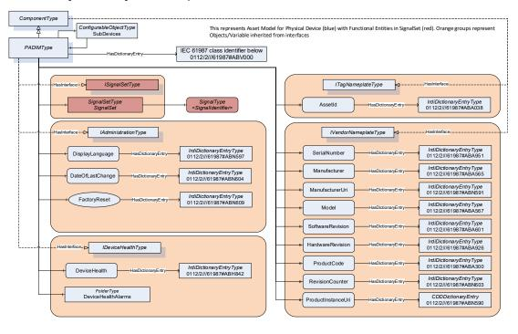
Figure 32: Extract from PA-DIM information model - references to IEC CDD
