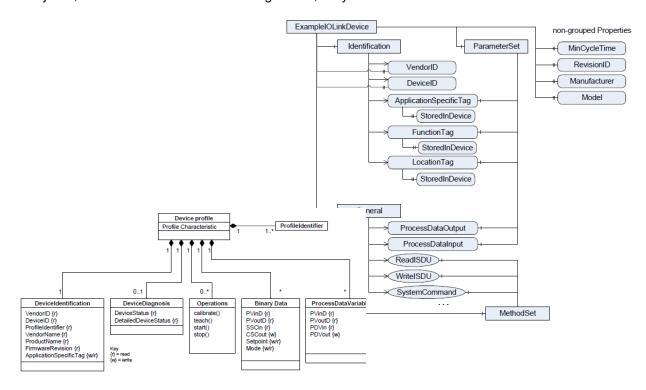
Figure 39: Basic structure of the IO-Link Common Profile and its mapping in the OPC UA Companion Specification
