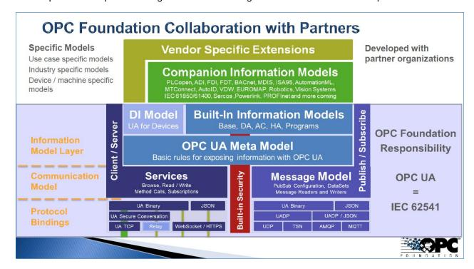
Figure 9: OPC Foundation Companion Specification developed in cooperation with domain partners
