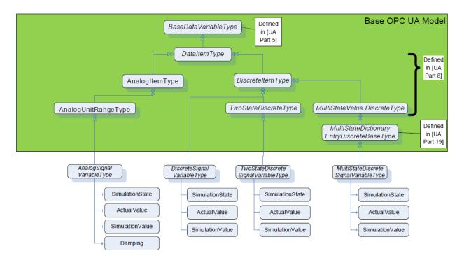
Figure 31: Extract from PA-DIM information model – analog and discrete values
