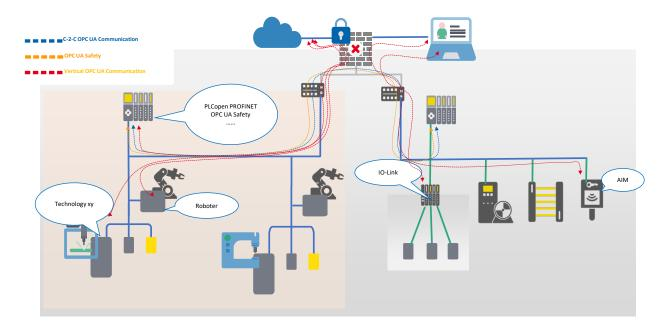
Figure 19: Different data sources connected with different technologies are provided by OPC UA
