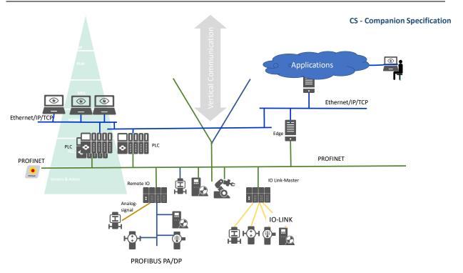
Figure 15: "Y"-oriented vertical communication in the automation system
