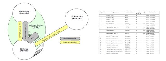
Figure 34: Parameter overview for PROFIdrive and its access paths
