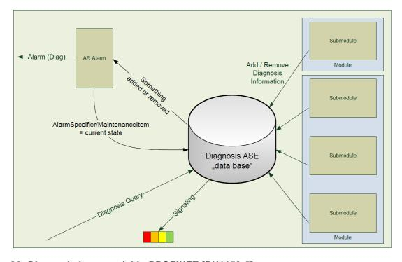
Figure 26: Diagnosis base model in PROFINET [PN1158-5]
