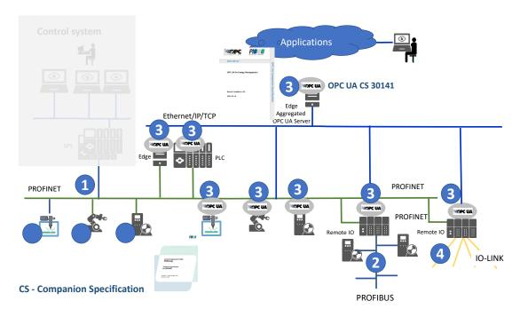
Figure 36: Typical integration variants of PROFlenergy in the communication network
