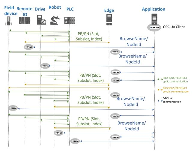
Figure 16: Communication principles in vertical communication
