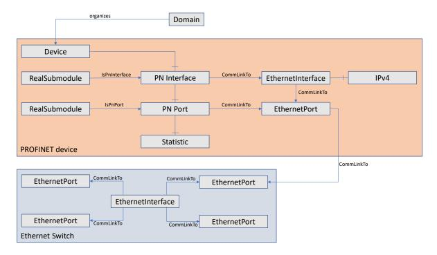
Figure 25: Physical network topology of a PROFINET network [PN1158-5]
