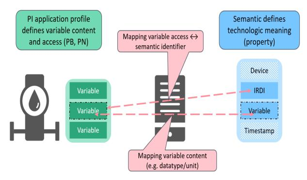
Figure 14: Mapping model between PI profiles and ID-based characteristic definitions
