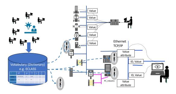
Figure 4: Use of a dictionary for the identification of field device parameters
