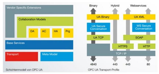
Figure 5: OPC UA layer model and transport profiles
