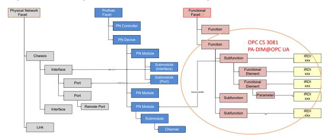
Figure 45: Characteristic integration with IRDI in the PA-DIM information model
