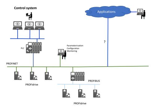
Figure 33: Typical integration variants of PROFIdrive devices
