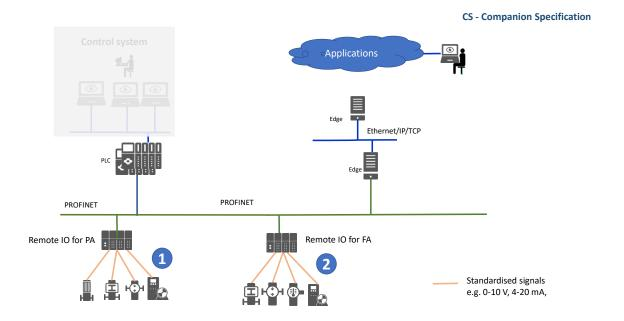
Figure 40: Classification of Remote IO for FA and PA
