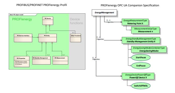
Figure 37: Basic structure of the profile and its mapping in the OPC UA Companion Specification
