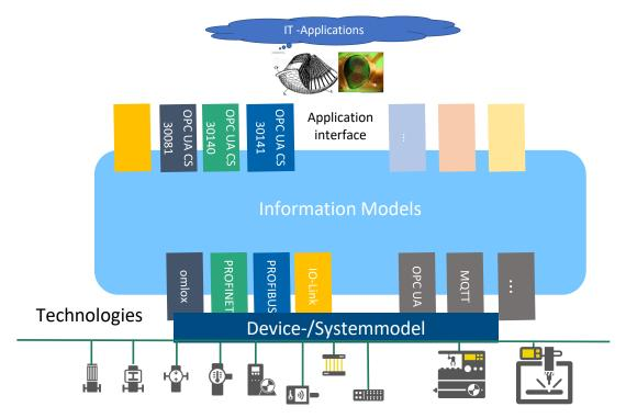
Figure 20: Information models provide cohesion between the different PI technologies
