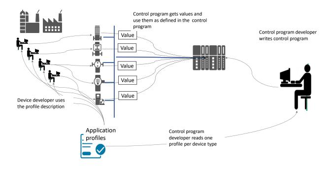
Figure 3: Profile-based approach to creating control programs
