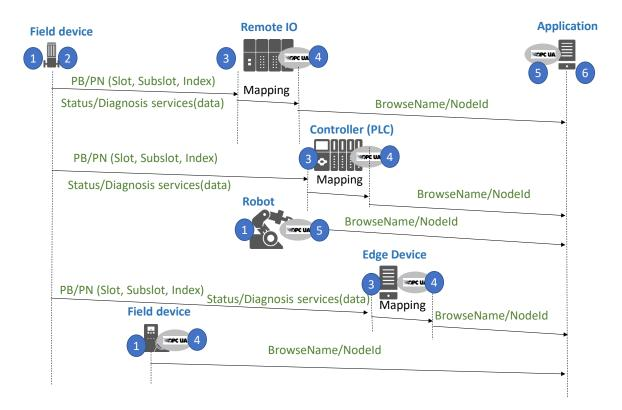
Figure 17: Data point addressing and diagnostics along the data path from the field device, drive, Remote IO or robot to the application
